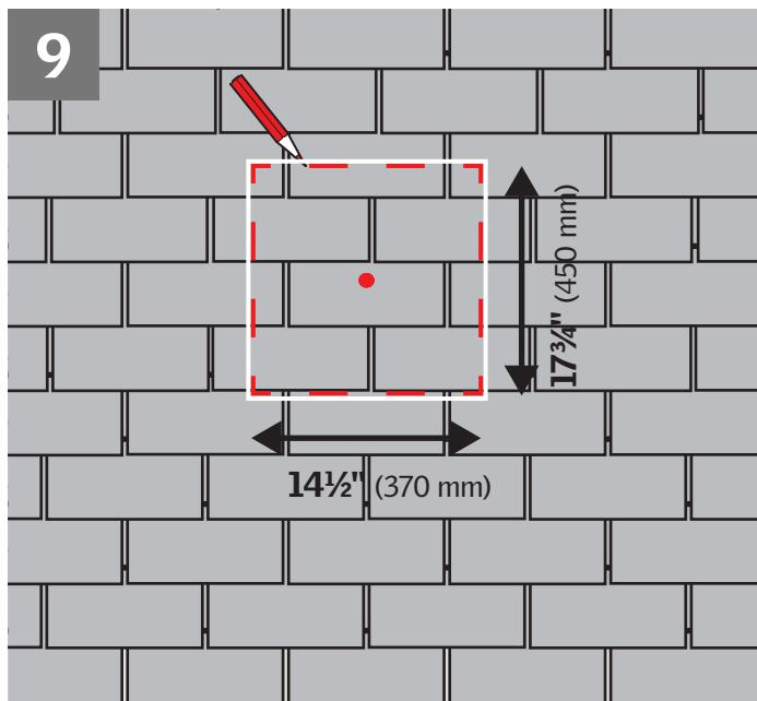
**ENGLISH:** Locate the nail indicating the center of the sun tunnel on the roof and mark rough opening.
