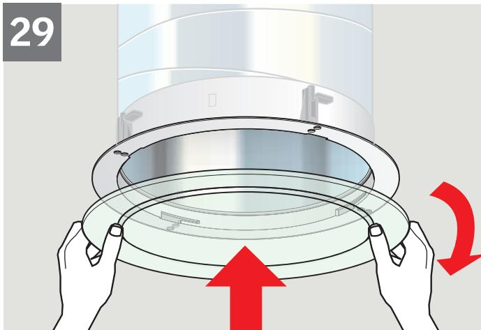
**ENGLISH:** Install the diffuser assembly by aligning the notches and rotate to secure.
