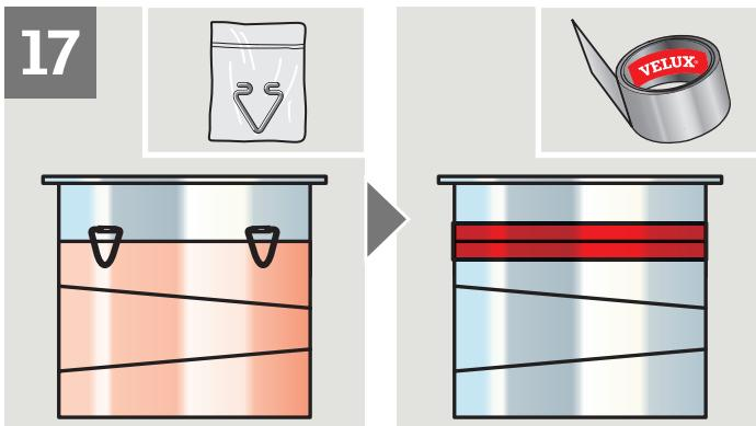
**ENGLISH:** Attach the upper elbow to the top collar. Secure joints with tunnel clips and tape provided.
