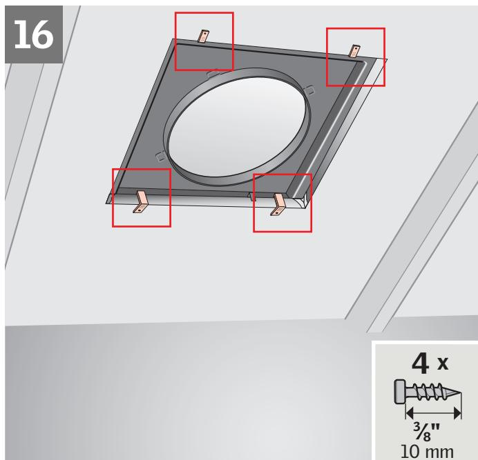
**ENGLISH:** Bend straps as shown and secure with the  $3/8"$  (10 mm) screws provided.
