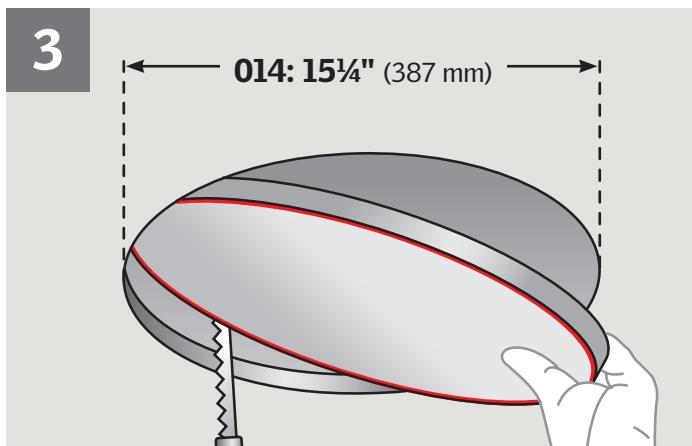
**ENGLISH:** From the inside, locate the nail indicating the center of the sun tunnel in the ceiling, mark circle and cut rough opening in the ceiling as shown.
