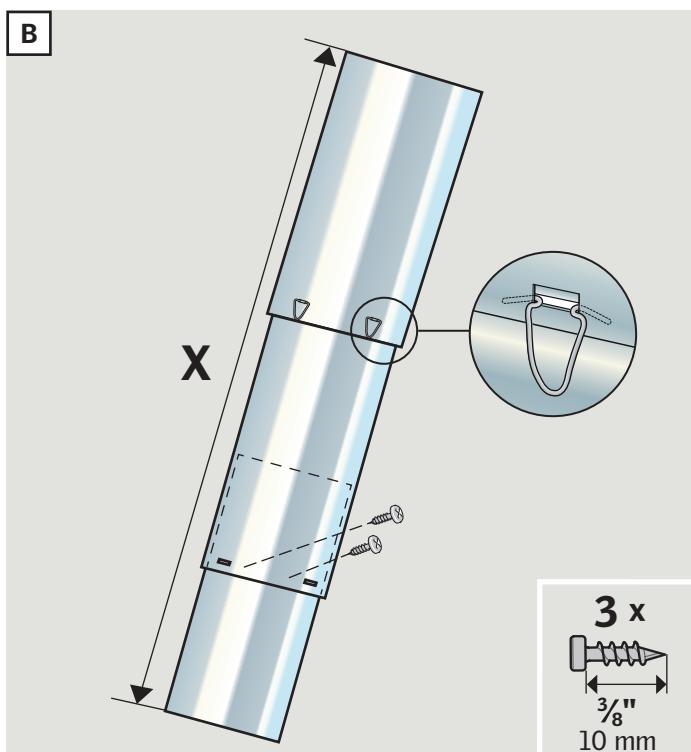
**ENGLISH:** With more tunnel sections, assemble the upper sections with the tunnel clips provided and reduce the length of the tunnel assembly by increasing overlap at the bottom. Secure the joint with three of the  $\frac{3}{8}$ " (10 mm) screws **B**.
