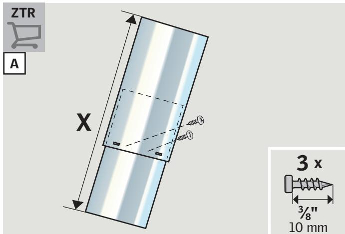
**ENGLISH:** With two tunnel sections, reduce the length of the tunnel assembly by increasing overlap. Secure the joint with three of the  $\frac{3}{8}$ " (10 mm) screws **A**.
