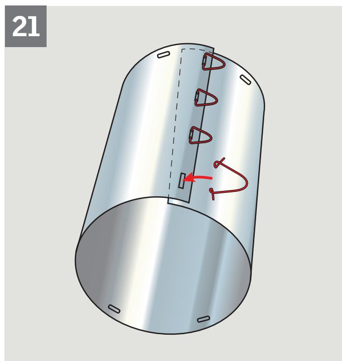
**ENGLISH:** Assemble the rigid tunnel sections with tunnel clips provided.
