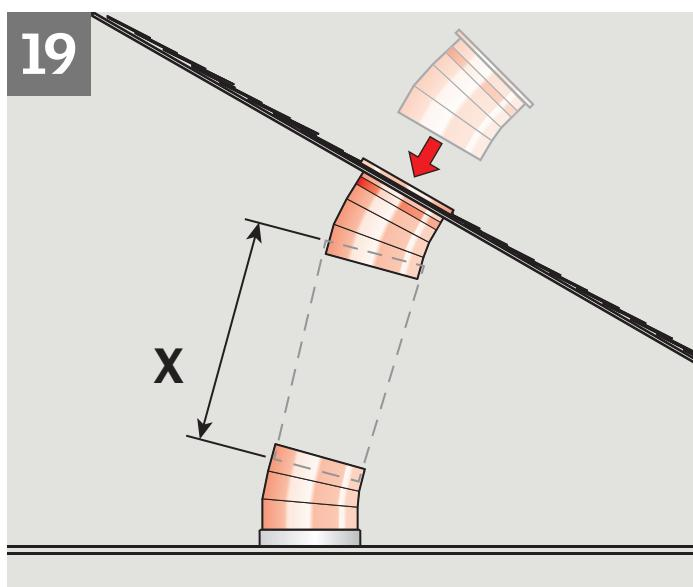
**ENGLISH:** Adjust the angle of the upper elbow so that it points directly against the lower elbow. Elbows can be damaged if excess force is applied.
