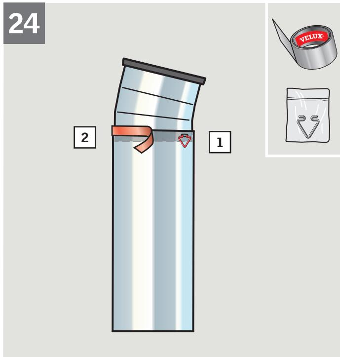
**ENGLISH:** Connect the rigid tunnel section with the upper elbow, fitting the rigid tunnel section to go on the outside of the upper elbow. Secure and tape joints with tunnel clips and tape provided **[1]**, **[2]**.
