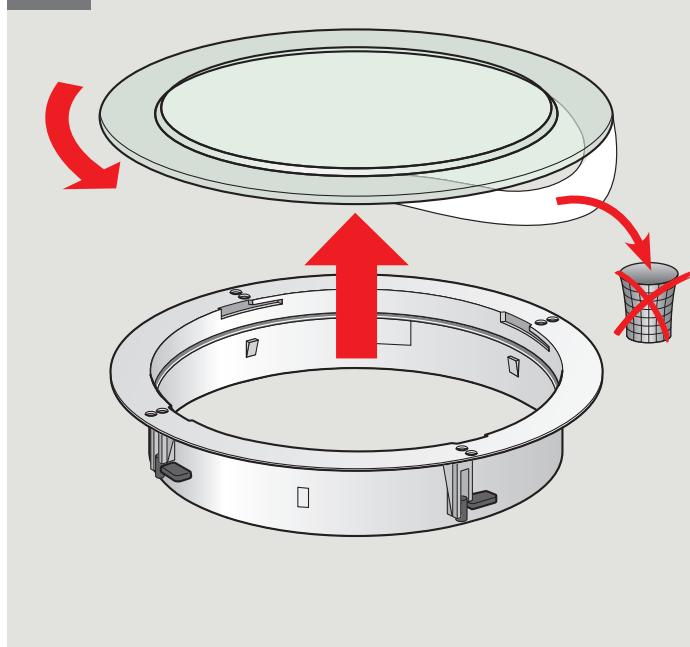
**ENGLISH:** Carefully remove the primary diffuser from the ceiling ring. Rotate the diffuser to disengage.
