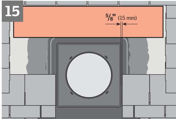
**ENGLISH:** Reinstall roofing material over the flange. Leave a  $5/8"$  (15 mm) channel for water to run off.
