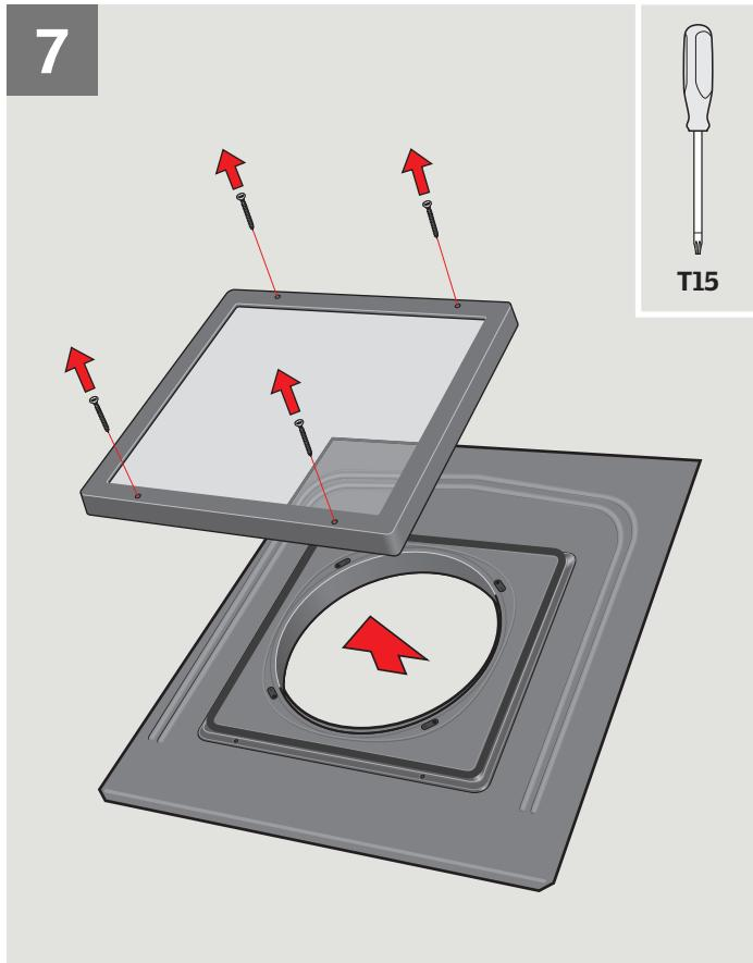
**ENGLISH:** Unscrew and remove lens from flashing.
